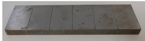
Figure 27-10 1018 CS depth sizing calibration standard
